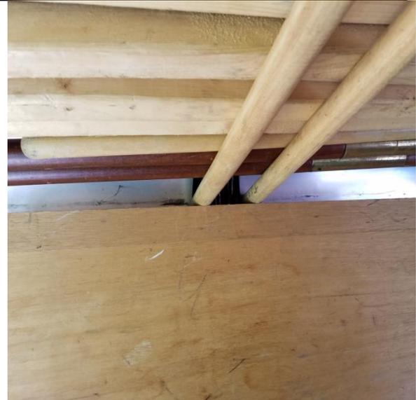
This part is critical. The staves used to support the tarp poles **MUST BE WEDGED BENEATH** the wiring harness. Be careful not to crimp or otherwise pinch these wires lest we lose our lighting system!
